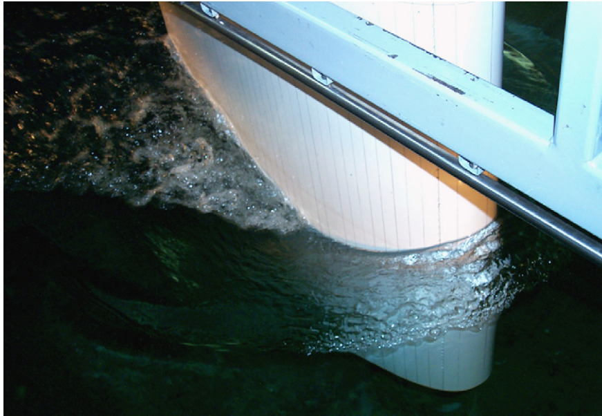
Fig. 1. Surface-piercing NACA24 foil at Fr = 0.37 .
